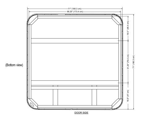
**NOTE: WATKINS WELLNESS** recommends that the SX be installed on a minimum 4" (10.2cm) thick reinforced concrete pad or structurally sound deck able to support the "dead weight" found in the spa specification chart. **IMPORTANT:** THE SX MUST NOT BE SHIMMED IN ANY MANNER.
