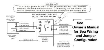
wiring access panel of the control box. A licensed electrician should install a four-wire electrical service (two line voltages, one neutral, one ground) from the main electrical service panel to the subpanel.
